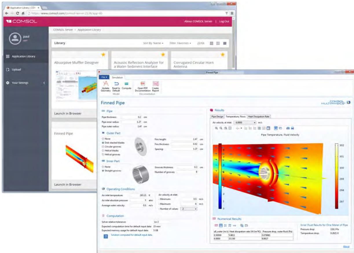
*The thermal properties of a finned pipe are derived from the results of a conjugate heat transfer simulation. The app user can change aspects of the design such as the arrangement of the inner grooves and outer fins.*
