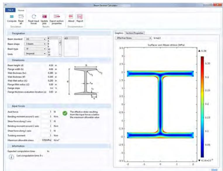
*With this simulation app users can test different beams, materials, and loads to analyze the resulting stress, strain, and displacement.*
