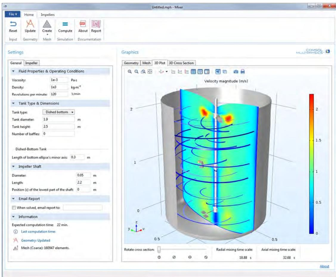
*This simulation app is intended for the simulation of mixers equipped with axial or radial impellers. For a given geometry, the application computes the efficiency of the mixing process. The vessels, which are available in three different shapes, can also be equipped with baffles and any of eleven different types of impellers.*
